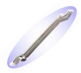
Adjust Spicer Easy-Pedal clutches with one hand and one tool. How? The end of the tool is placed into the clutch inspection hole, with the socket positioned on the adjusting bolt. Depress and turn the tool to adjust the clutch. Simple - and it only takes one hand!
